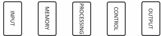
Figure 1. The five primary components of a computer system: the input, output, memory unit, control unit, and central processing unit. Their relations in terms of control and information flows are not shown explicitly here. More details can be found in computer-science textbooks, e.g. [47].
